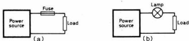
Fig 1. If a response time of several tenths of a second is tolerable, circuits can be protected with a fuse as at (a), or with an incandescent lamp as at (b). These protectors will work on either ac or dc
